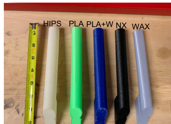
Figure 2. Examples of printed tensile bars (Figure 1) in five different materials.
